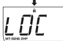
To unlock, turn the controller off, and then turn it on again with the key **F** pressed. Keep the key pressed until the message **LOC** is displayed. After releasing it, the message **Off** will be displayed.
