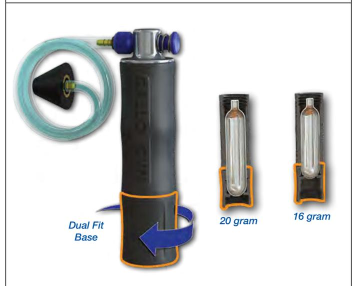
2. While holding the tool with the cartridge in an upright position (the tip of the cartridge facing upward), screw in until the cartridge just contacts the puncture pin, and then quickly and firmly twist it in until it stops. This will prevent loss of CO<sub>2</sub> gas.
