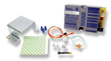
The Robertshaw® 780 Series Pilot Controls Uni-Kits® feature a flame sense circuit that will work equally well on a one rod (local sense) or a two rod (remote sense) application. The automatic recycle features assure that, in the event of flame failure, main gas is disabled and the spark repetition sequence is restarted until pilot gas is ignited. Only after pilot ignition has been re-established can main gas be returned to the burner.
