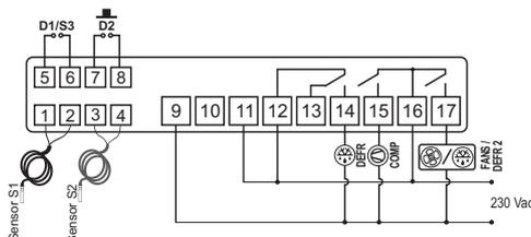
The sensor S1 must be in the ambient. The sensor S2 must be placed in the evaporator through metallic cramp.
